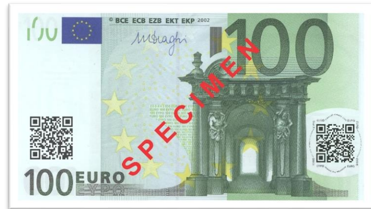
Proposed design for €100 CryptoNote with foil patch removed to reveal private key QR code.
